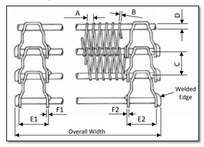
**NOTE:** When measuring pitches A & C, it is best practice to measure over 10 pitches and divide by 10 to obtain the average pitch.
