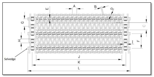
**NOTE:** When measuring pitches A & C, it is best practice to measure over 10 pitches and then divide by 10 to obtain the average pitch.
